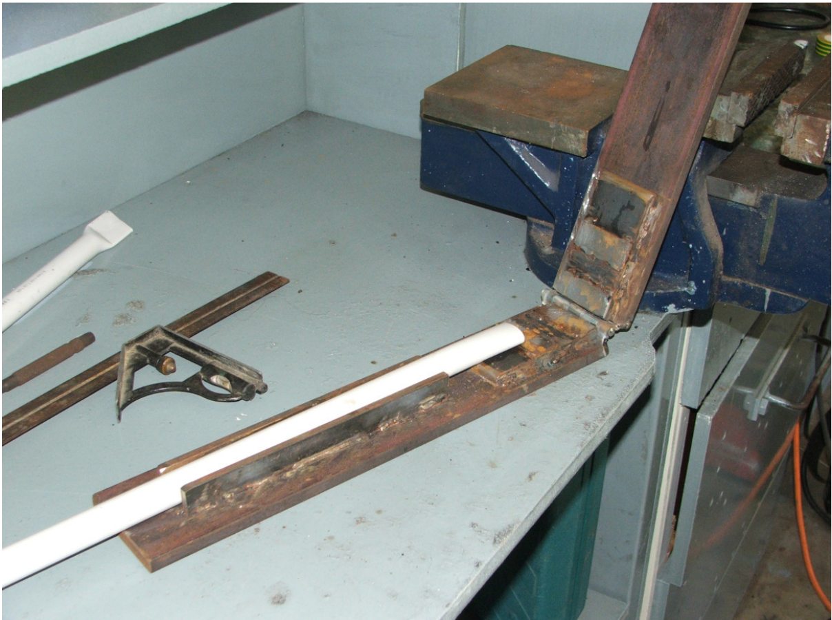
Pic 3 – End flattening jig.
