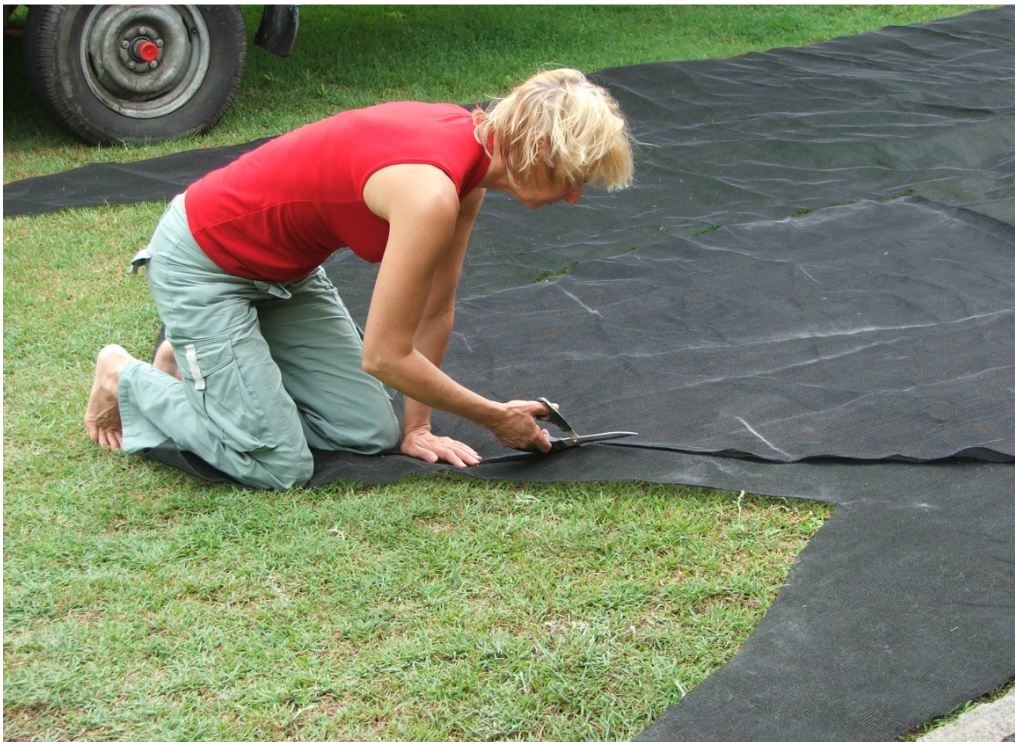
Pic 13 - Cutting shade cloth into triangles. Sown using sail cloth thread on a home sewing machine.
