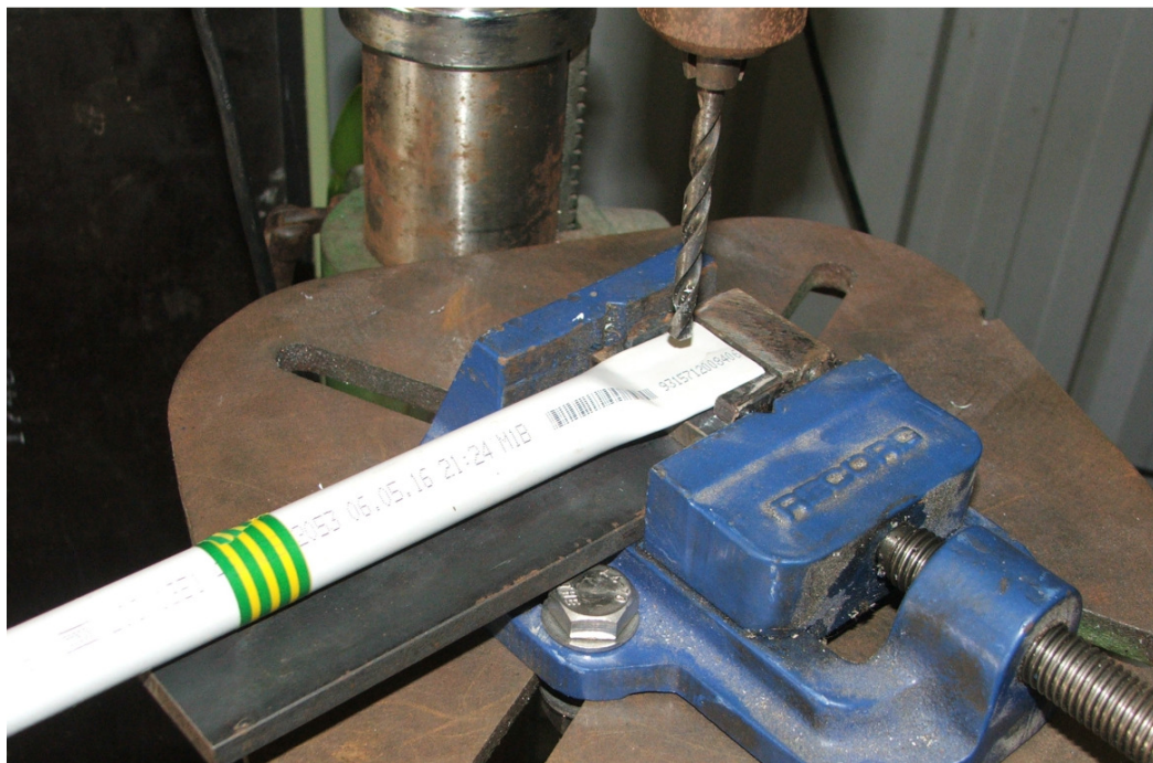
Pic 7 – Drilling all one end of the struts.
